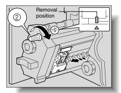
**12** Grasp both sides of the staple cartridge holder, lift it up, and then pull it out.
